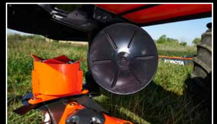
The machine is standard equipped with two swath discs, allowing a swath width of 7'3"-7'10" (2.2-2.4m).
