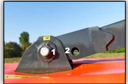
Two mounting options for optimal overlap with a front mounted machine.
