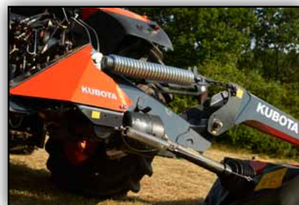
The large compensating spring ensures excellent flotation across the full mower width.
