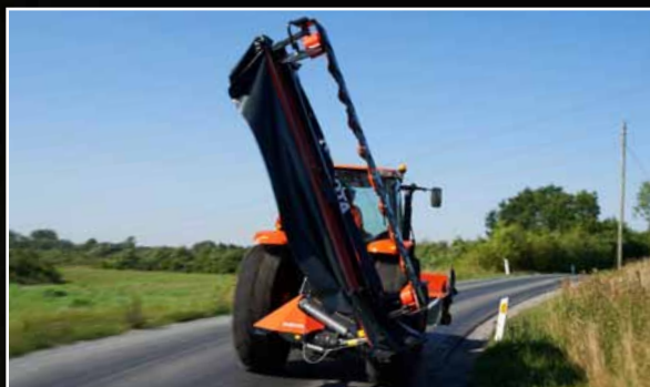
125° vertical transport position for excellent weight distribution.
