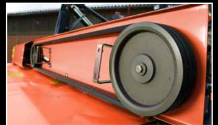
By switching driveline pulleys changing from standard PTO speed of 1000 rpm to 750 rpm is possible.
