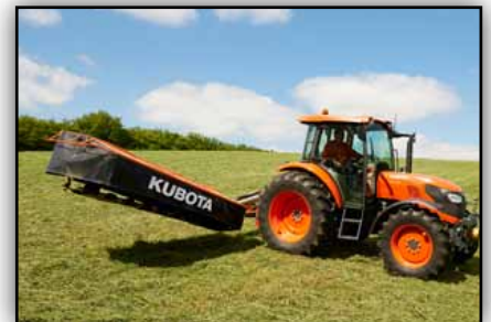
Lift on headlands via a hydraulic cylinder – no use of the 3 pt hitch is needed.
