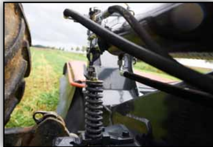
When encountering an obstacle the NonStop BreakAway system protects the cutterbar by swinging it back and up.
