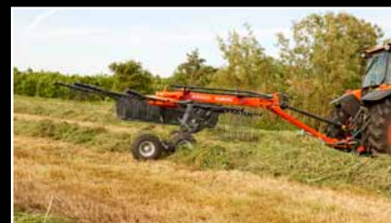
RA1042T and RA1047T can conveniently be raised up to a height of 1'7" (50cm) from the tractor driver's seat.
