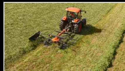
RA1042T designed for low hp tractors, while still delivering 13'9" (4.2m) working width.
