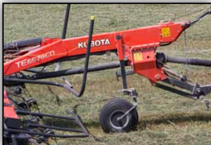
A third wheel allows for better tracking and more accurate tedding action. This wheel also helps adjust the tedding height.
