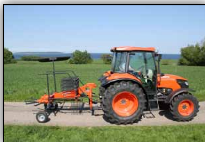
RA1035 - For reduced transport and storage width, tine arms can be placed on the carrier frame.
