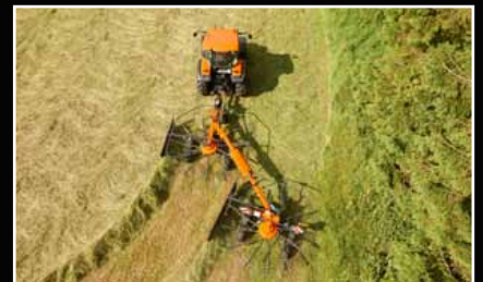
Both rakes are capable of placing small tight swaths for hay crops.
