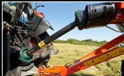
Wide angle PTO shaft - for increased maneuverability.
