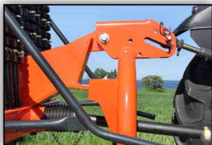
A pivoting 3-pt headstock ensures perfect ground following.
