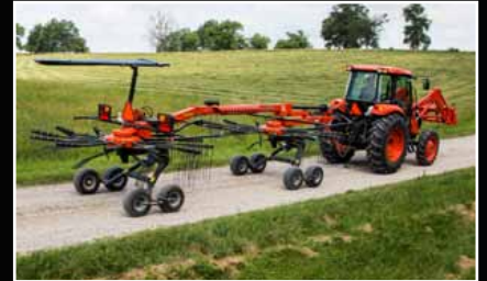
Pulled axle suspension for smooth running and reduced power requirement.
