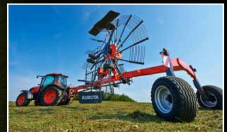
Active wheel steering for improved manoeuvrability in combination with large wheels for reduced compaction.
