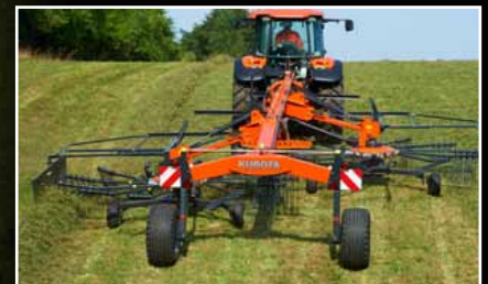
The side delivery concept allows you to collect crop from 49'3" (15m) into a single swath.
