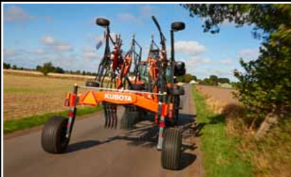
With tine arms removed, transport is as low as 11'4" (3.45m).
