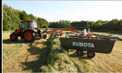
With 1'8" (50cm) lifting height, swaths are easily crossed.
