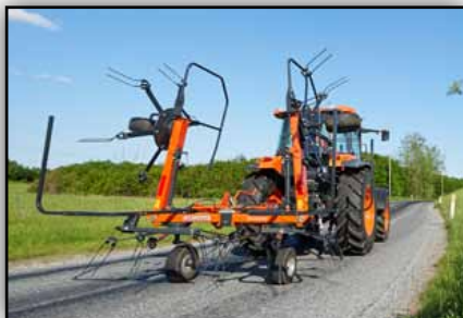
The tines are automatically leveled for added ground clearance when folding into the transport position.
