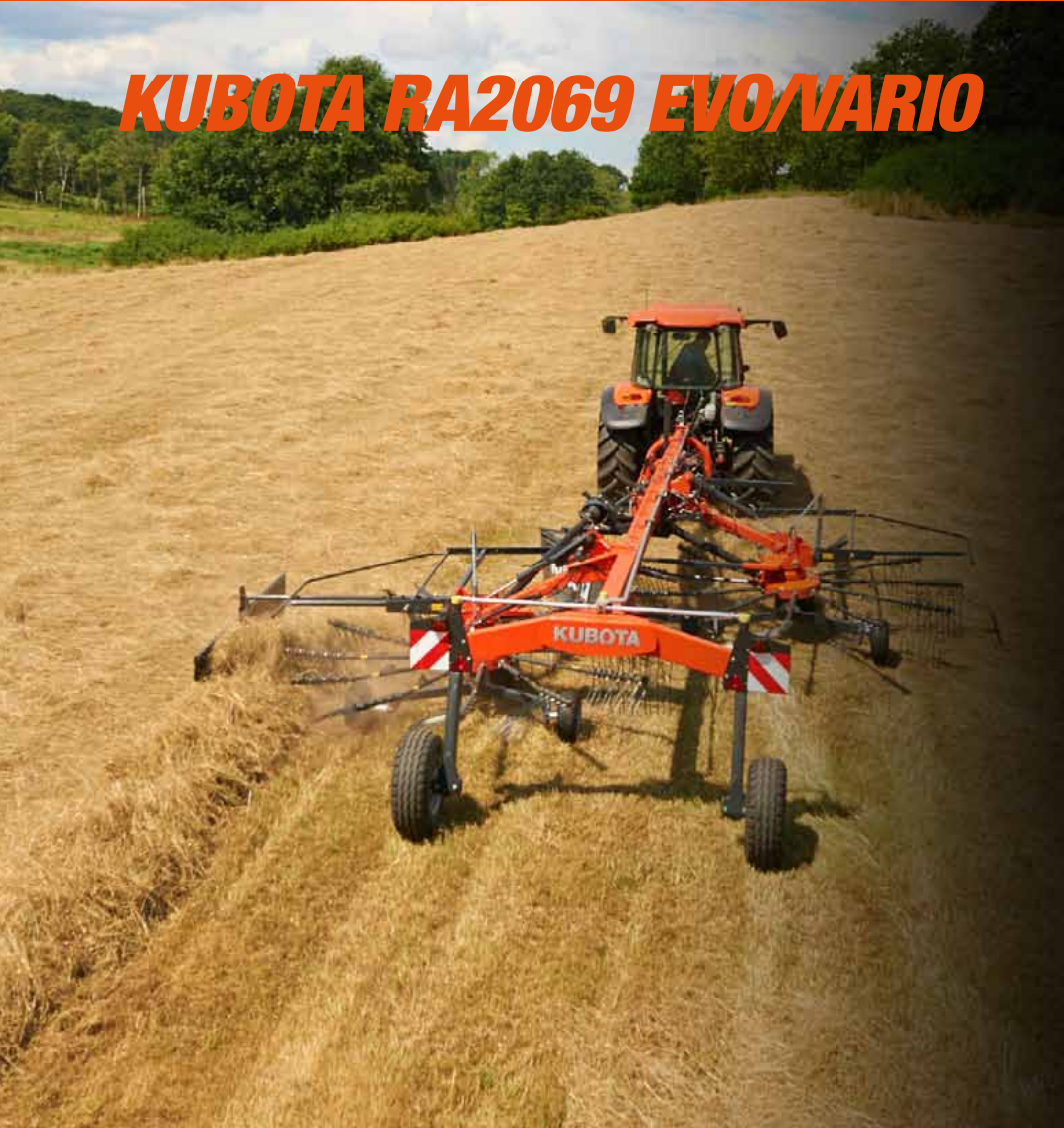
Generous overlap between rotors ensure clean raking.
