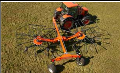
The ability to make sharp turns up to 80° and the cross stabilizer in the headstock are unique Kubota features.
