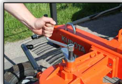
Easy setting of correct rotor height.
