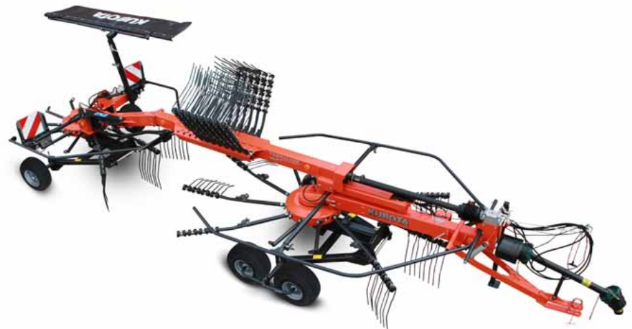
Wide angle PTO shaft - for increased maneuverability.
