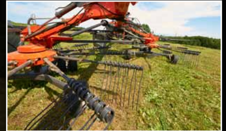
Generous overlap between rotors ensure clean raking.
