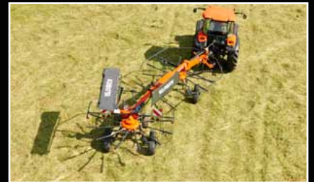
SideShift to the left - raking without driving on unraked crop.
