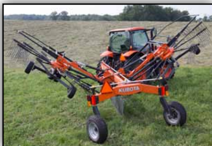
The ability to make sharp turns up to 80° and the cross stabilizer in the headstock are unique Kubota features.
