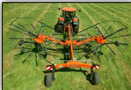
The hydraulically adjustable rotors can be set at 20'4"-23'11" (6.2-7.3m)...
