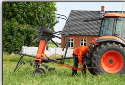
Pull type drawbar. Easy to attach.
