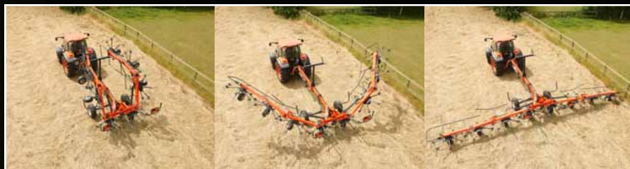
Fast and efficient conversion from transport to working position.
