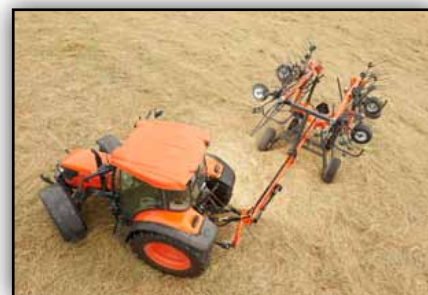
80° turning angle ensures excellent manoeuvrability.
